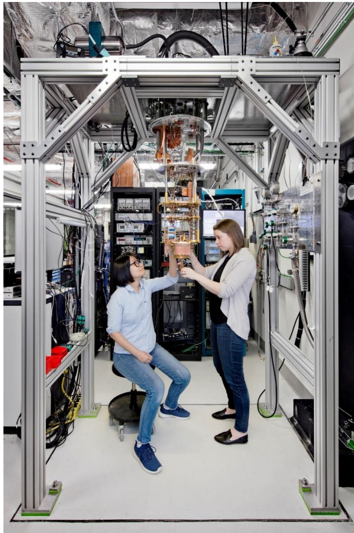
FIGURE 3: IBM Quantum Computing Scientists examine the hardware inside an open dilution fridge at the IBM Quantum Lab at IBM's T. J. Watson Research Center in Yorktown, NY. (Source: IBM Research)
